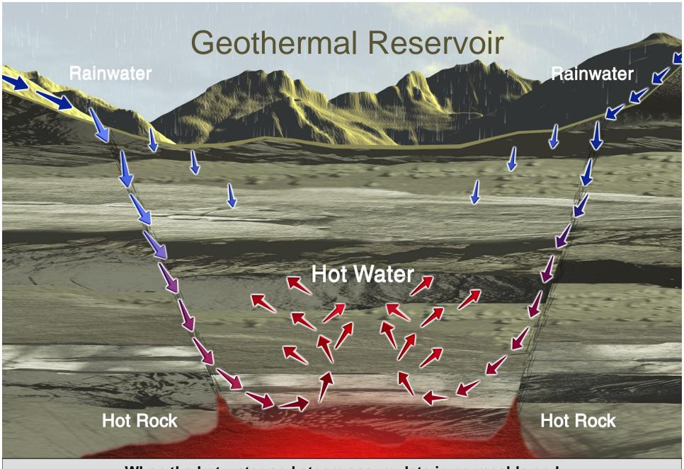
When the hot water and steam accumulate in permeable and porous rock, a geothermal reservoir forms.
