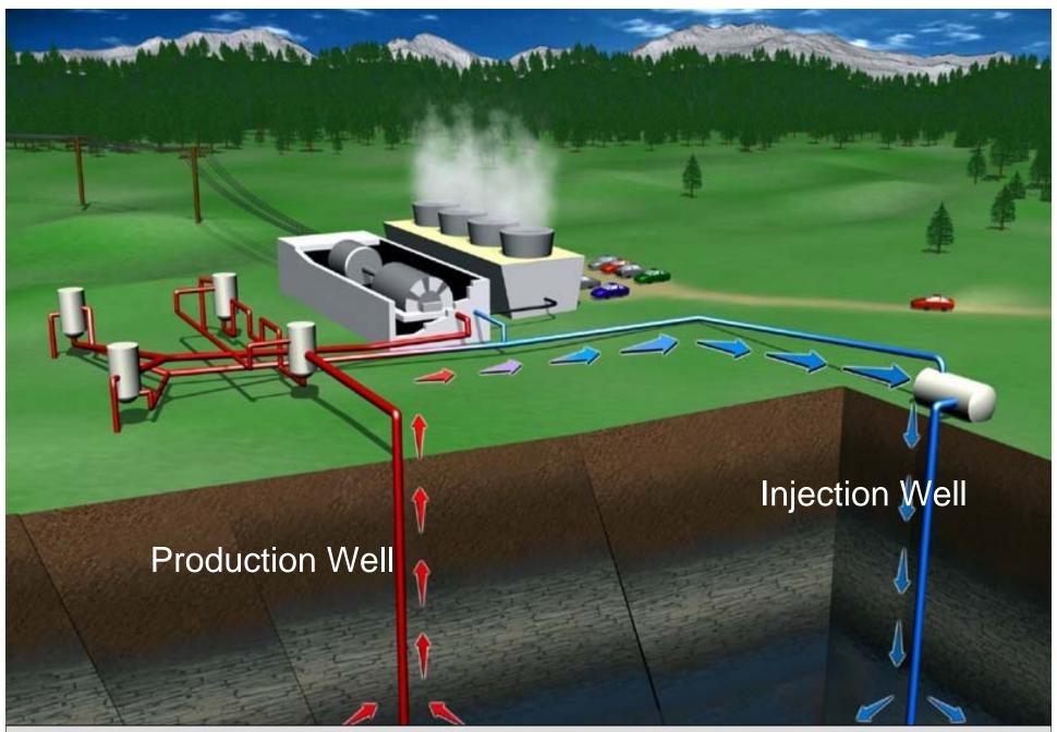
Natural steam from the production well powers the turbine generator. Condensed steam and unused hot water are injected back into the reservoir, thus sustaining production.
