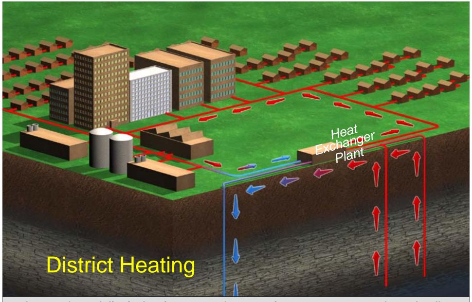
In a geothermal district heating system, hot water from one or more geothermal wells is piped through heat exchanger plant to heat city water.
